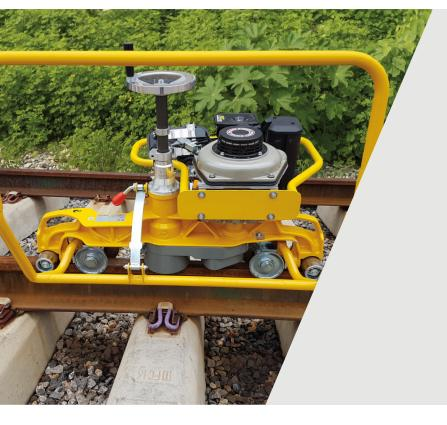
The Gamma Grinder has been designed to fully grind the rail head after welding. Like all of Pandrol's grinding machines, it combines power and reliability with ease of use.
