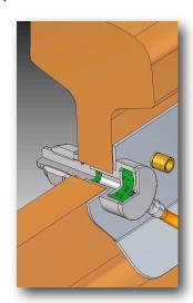
The accelerometer is complementary to the strain sensor and indexable at 45 degree increments in the sensor body so that it can still be positioned in
