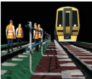
Barrier set at 4ft (1.25m) from running rail for lines speeds up to and including 100 mph
