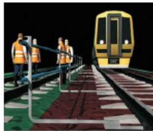
Barrier set at 6ft 6" (2m) from running rail for lines speeds over 100 mph
